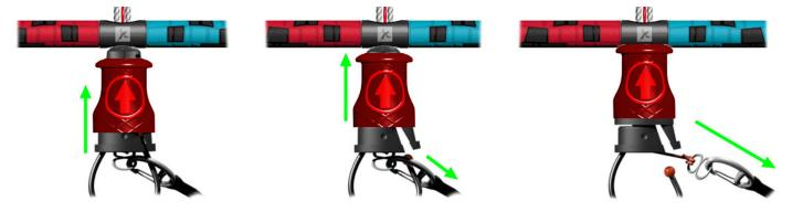
To rig in 'suicide' mode you must clip the karabiner over the chickenloop and into the leash ring. Even if you have dropped the bar or are riding unhooked your safety will not work fully until the *Pro-cuff QR* is activated.
