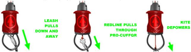
Advanced riders who are willing to trade maximum depower for faster relaunch can choose to rig the suicide leash option, shown below. When attached as shown below the kite will remain powered even with the bar unhooked. Only when the *Pro-cuff QR* has been pushed upwards and activated will the kite depower and fall from the sky.
