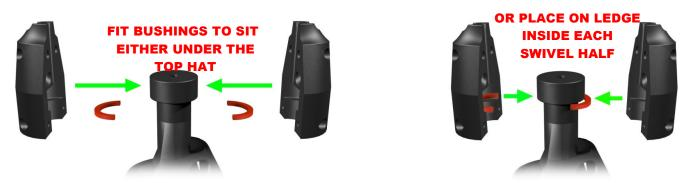
To replace the swivel bushings, remove the four screws that hold the swivel together, prise out bushings with a flat bladed screwdriver and then reassemble as shown below.
