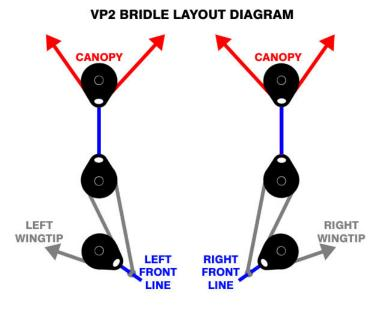
The Nemesis HP front bridle has user-replaceable heavy duty inserts fitted at two points; within the VP2 bridle section, (detailed in grey), and also for the upper floating pulleys (detailed in red). Should these become worn, simply undo the retaining loops at either end and fix in place a replacement set. It is recommended that you replace both sides, left and right at the same time even if only one side is showing wear.
